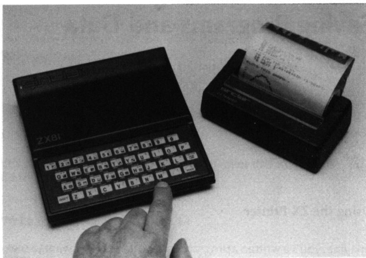
The ZX81 and the ZX Printer, designed especially for use with Sinclair personal computers
